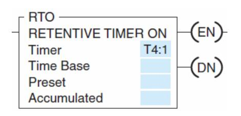
This timer must be accompanied by a timer reset instruction to reset the accumulated value of the timer to 0.
