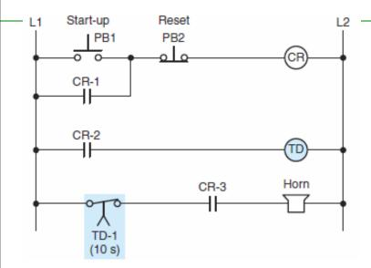
Hardwired Relay Circuit – warning horn sounds for 10 seconds whenever start button is actuated.
