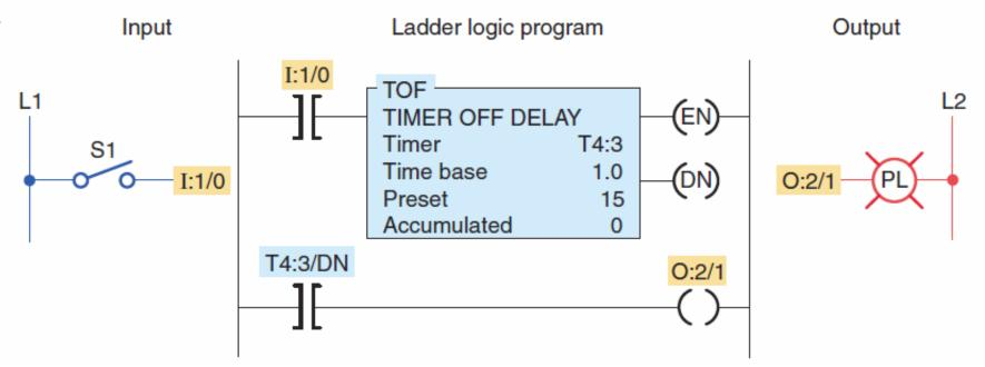
When the switch is first closed the lamp is switched on.
